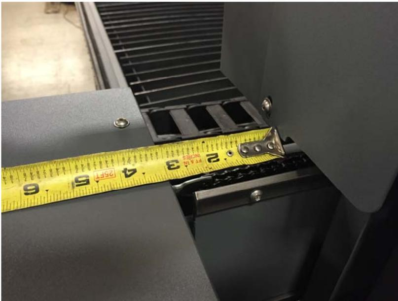
Repeat steps 2 – 6. 40" works well for a 4x8 machine. 50" works well for 5x10 and 6x12.
