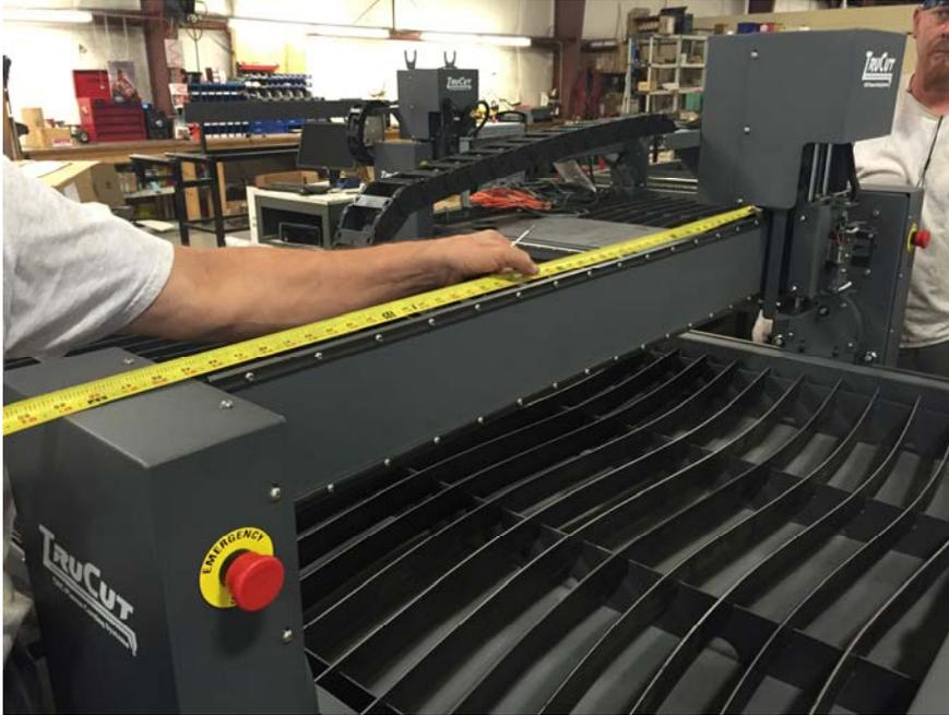
Your machine should now be calibrated. If you are still getting inaccurate motion, check set screws on belt pulleys and sprockets. If a set screw is loose, it will feel like backlash in the system and can cause inaccurate motion.
