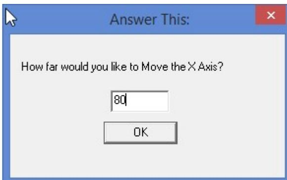
6. If the axis is calibrated correctly, it will move to the distance you told it to move. Re-measure from the same points that you previously measured and note that measurement. The actual distance moved will be this measurement minus 10". If you told it to move 80" and you are now measuring 90.25", you moved 80.25".
